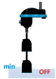
Low level stops the pump
